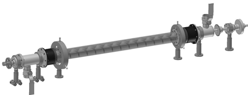
Fig. 24. Sketch of the high temperature rotary kiln reactor for char activation. The operation temperature is 950°C with steam flow and the char throughput amounts to max. 1 kg/h.
